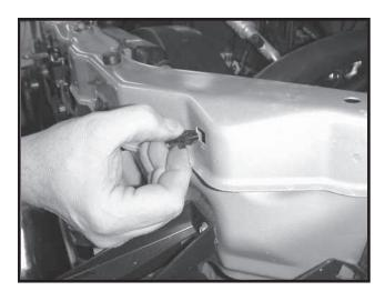
**3.** Release four plastic fasteners from vehicle and put back in grill for later installation.
